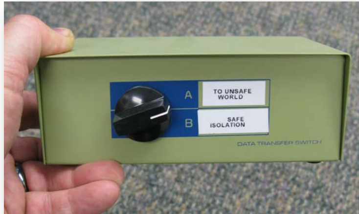
Figure 39 - Front view of a commercial RJ45 switch box with labels added by the authors.
