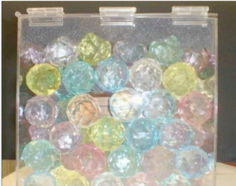
Figure 28 - An example of a beads-in-a-box seal. The “beads” in this case are multi-faceted silicone balls. Any access to the box disturbs the balls, which can be easily detected with a blink comparator.
