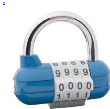
Figure 15 - A commercial 4-digit combination lock that uses alignment slots. Each of the 4 disks has an internal slot. Only when the slots align (at the correct combination) will the lock open. This type of design could be used to increase the number of possible "combinations" for the Magic Slate seal, though a more secure design would be necessary than exists on this inexpensive bicycle lock.
