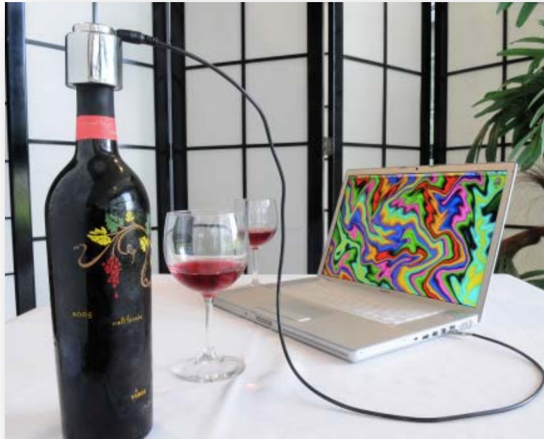
Figure 33 - Wine authenticity prototype. The inexpensive, reusable silver cap on top of the wine bottle can determine if the wine bottle has ever been opened (using an anti-evidence seal), and if it is an authentic bottle (using a virtual numeric token). The cap is connected to the Internet using a cable to “call-in” the virtual numeric token.
