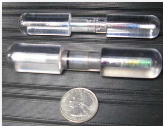
Figure 18 - Mock-ups of the Glass and Powder Seal, with powder bands of varying color, composition, and particles shown.
