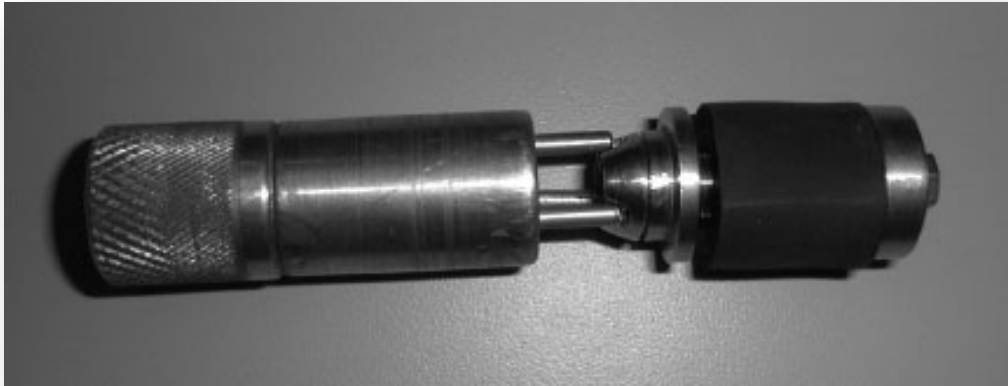
Figure 22 - One implementation of the Plug Seal. The “wrench” at the left is used to rotate the nut at the left end of the plug after the plug has been inserted into a bolt hole. This compresses the rubber, causing it to expand inside the bolt hole. There are other possible mechanisms for compressing the rubber as well.
