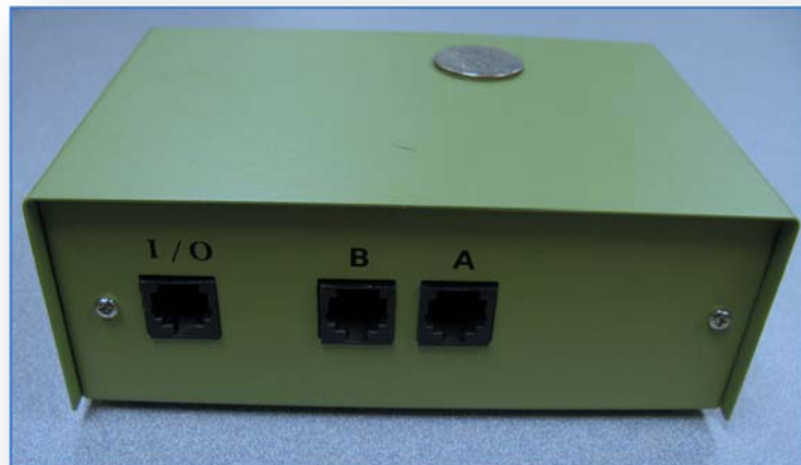
Figure 40 - Rear view of the switch box. A cable is used to connect the I/O port to the Ethernet router, while another cable connects the A port to the computer's Ethernet port. No cable is connected to B for this application.
