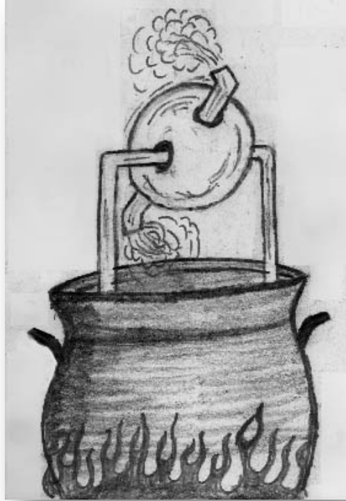
Figure 31 - Hero's Aeolipile. of Alexandria invented the world's first steam engine, called an aeolipile.[38] Water was heated such that the resultant steam could pass through pipes into a hollow sphere. The sphere had two jets through which the steam could escape, generating thrust that caused the sphere to rapidly rotate about its axis. It's not clear if Hero's device was ever actually built. In any event, the aeolipile was never considered anything but a toy until more than a thousand years later.
