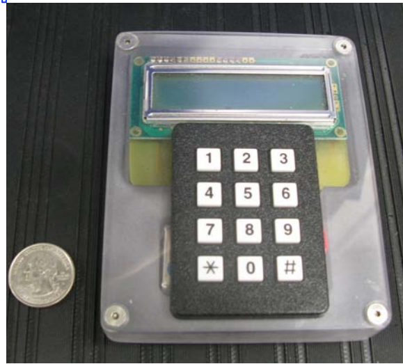
Figure 5 - A prototype device for computing the 2-letter hash algorithm after the secret key and the elapsed time are entered.
