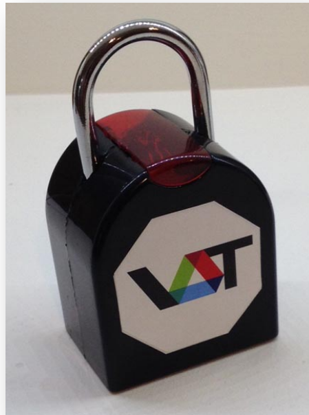
Figure 1 - One of our working Time Lock prototypes. The shackle and some of the interior is metal, while the outside is plastic. The prototype shown is 6 x 4 x 10 cm, much larger than is necessary. The prototype uses less than $20 of parts (quantities of 1).
